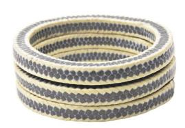
properties at elevated operating temperatures. It is suitable for a wide range of chemical media including water, steam, salt solutions, alkalis, organic solvents, mild acids, hydrocarbons and moderate chemical services. Most suited for rotary and plunger pumps.
