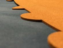
WCM1028 is a firm rubber/cork material suitable for medium bolt pressure with good flexibility and resilience.
