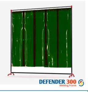
The wider frame dimension makes the Defender 300 a step up from the 100 and 200. Included with the kit is a pack of EN1598 welding strips, available in red or green. These consist of 5 strips that fasten together by click studs to its neighbouring strip, before attaching via curtain rings to the header rail.
